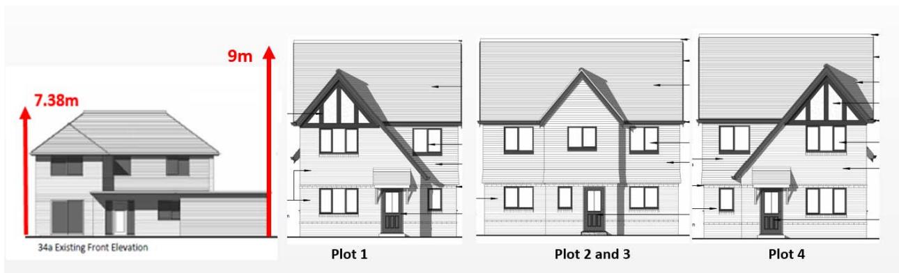
Figure 9 Comparison of elevations of existing dwellings at No. 34a and proposed dwellings
